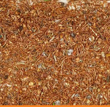
Output material: Non-ferrous fraction Bulk density: 3,00 t/m³
