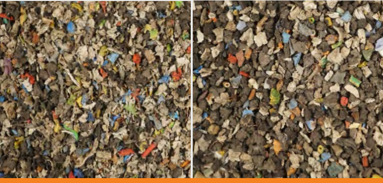
Output material: Light fraction Bulk density: 0,44 t/m³
