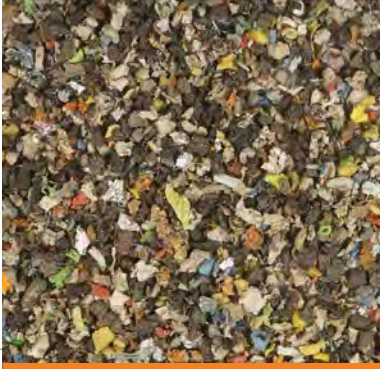
Output material: Plastics Bulk density: 0,49 t/m³
