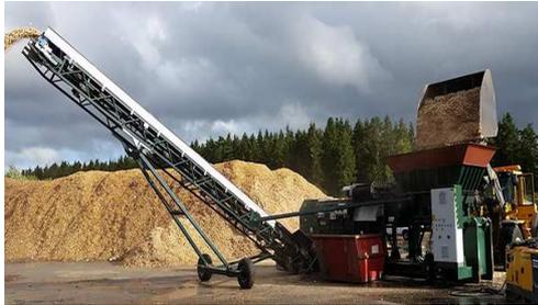
The integrated bunker enables material to be loaded continually using wheel loaders; the permanent magnetic overband separator cleans tramp iron; and the eddy current separator separates aluminum parts effectively from the other material. The whole unit can be moved with a crane hook, giving the customer a highly mobile application that enables wood chip to be produced as efficiently as possible.
