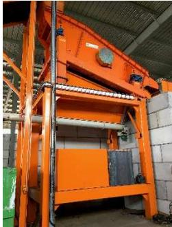
The unique structure of the resonance system makes it possible to adjust the oscillating behavior of each individual crossbeam and ensures that the system continues to perform even at steeper gradients – for blockage-free screening perfectly tailored to the task at hand.
