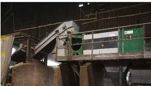
Fig. 8: Permanent magnetic separator, feed chute, and centric eddy current separator for cleaning waste wood
